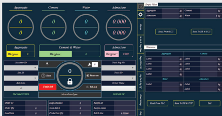
SCADA Main Screen (Dial View)
